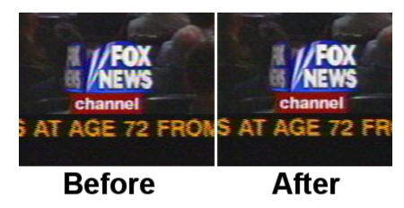
If you have vertical blanking information or crawls which constantly change in each frame, block them out with the **Mask** tool. This improves compression ratios.
